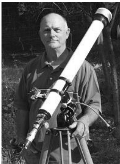
Figure 7: Darrell Grisham used a modified 1960's 3 inch Tasco telescope to make startlingly precise and accurate measurements of double stars.
